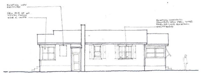
Proposed Window and Door Replacement North Elevation
