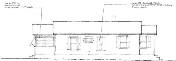
Existing Window and Door Replacement South Elevation
