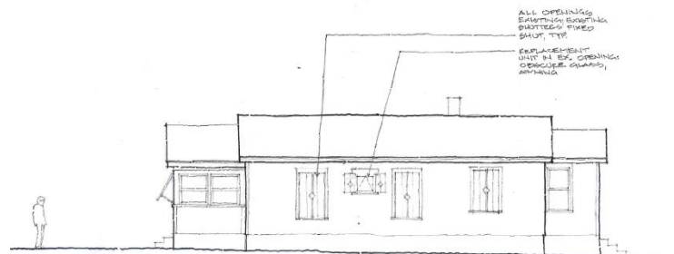
Proposed Window and Door Replacement South Elevation
